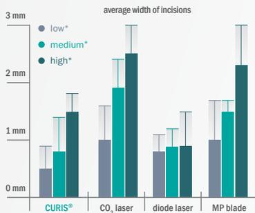
**Fig. 2:** Comparing the average width of incisions produced by different instruments at different energy levels
