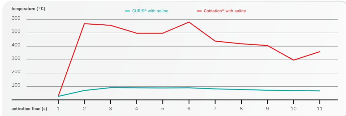
Fig. 10: Mean temperatures (°C) of a series of measurements using CURIS® with RaVoR™ bipolar electrode and Coblation® \*<sup>2</sup>
